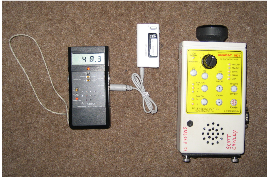
Figure 6: Recording Equipment used during detector surveys (L-R Pettersson D240x Time Expansion detector linked to Creative Nano Plus Mp3 recorder, Anabat SD1 Bat detector)
